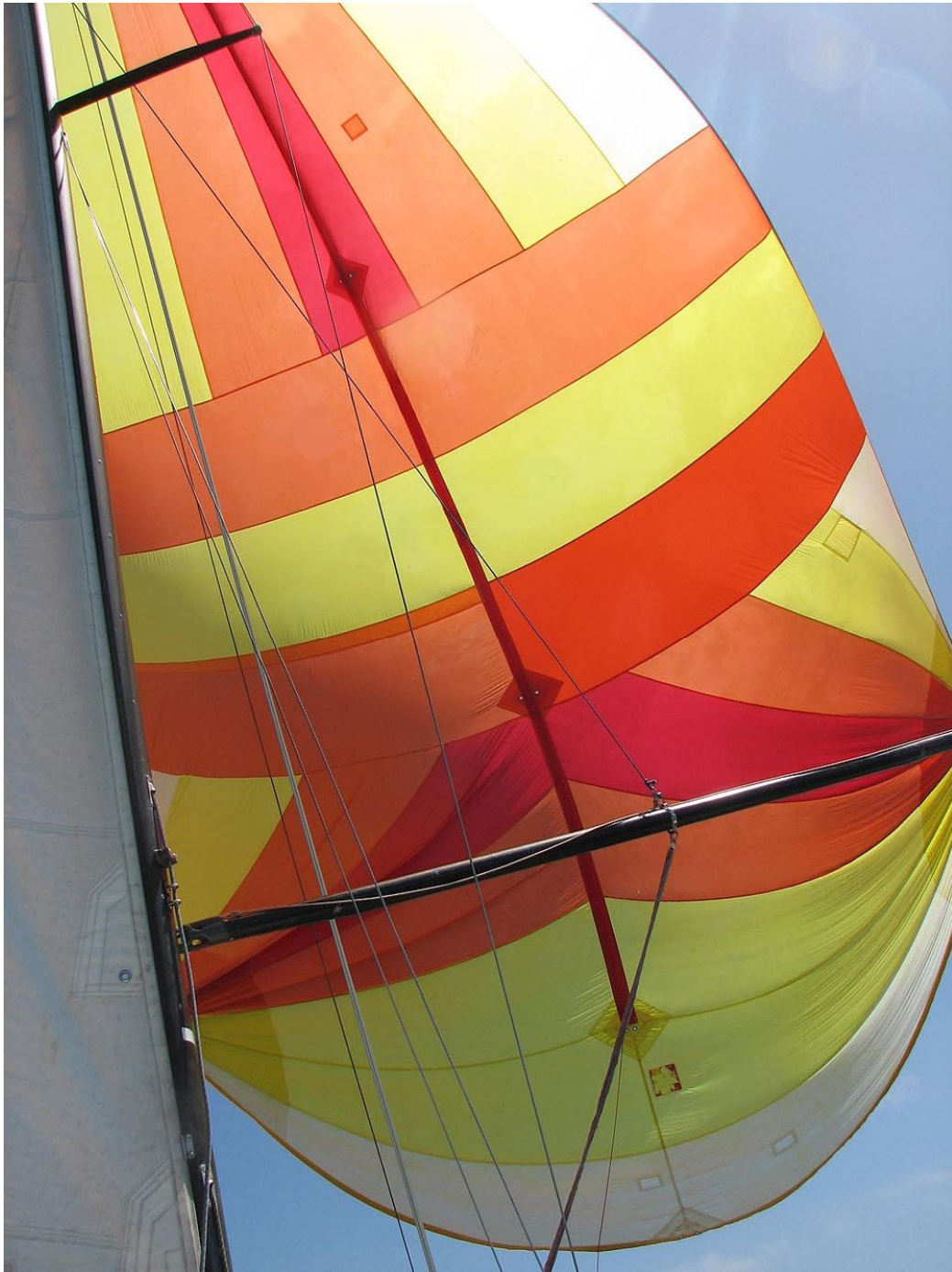
Merit 25 Twilight Zone sailing under full spinnaker (thong-off mode). The thong is lead through the nylon tube sewn vertically down the centerline of the sail, with patches and grommets to help transfer the load of the thong to the nylon sail. The thin line exiting the bottom patch is the thong line.
