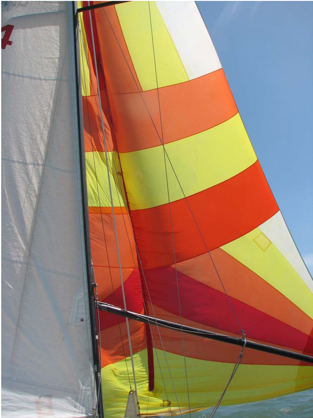
Merit 25 Twilight Zone sailing under spinnaker in thong-on mode. The thong has been tensioned, drawing the sail together along the centerline. Note that the sail shape has changed considerably, reducing power. The tensioned thong line, lead to the deck at the bow, helps to reduce the sail's lateral oscillation.
