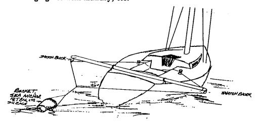
Boat will probably require jibs wing and wing for balance downwind.
